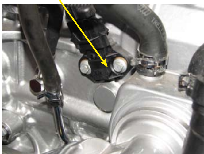
Lube Engine oil Temperature and Pressure sensor
