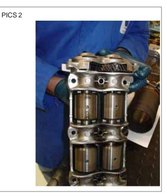
It is possible insert the tool into either couple of holes
